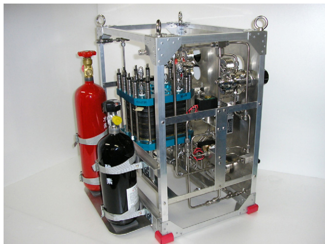
Fig. 3. A photograph of the fuel cell stack installed in the reactant supply subsystem.
